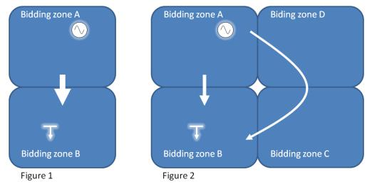
In figure 1, the bidding zones A and B are interconnected in a radial way. Just like the Danish-German AC border, there is a one-to-one translation from the scheduled power exchange between those bidding zones into a physical cross-border flow on the lines. Translated into the flow-based parameters, this means the interconnection has a PTDF = 1. With the general flowbased equation being:
